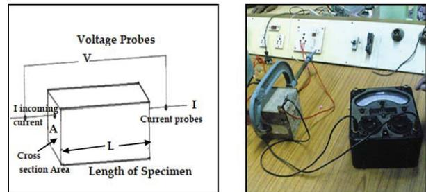
**Fig. 2: Schematic Diagram and Test Setup for Electric Resistivity**
